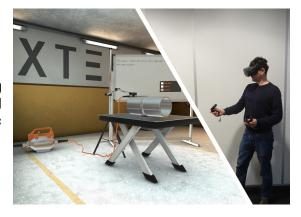
Each exercise is built to include all the preparation phases: choice of film, IQI, and choice, positioning and orientation of the source as well as setting the current and expose time of the shot.
